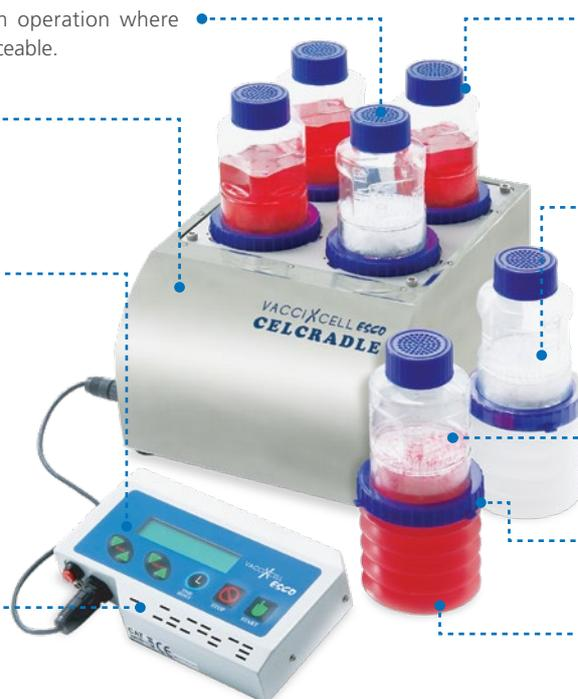
Bottle cap is integrated with 0.22µm ventilation filter
